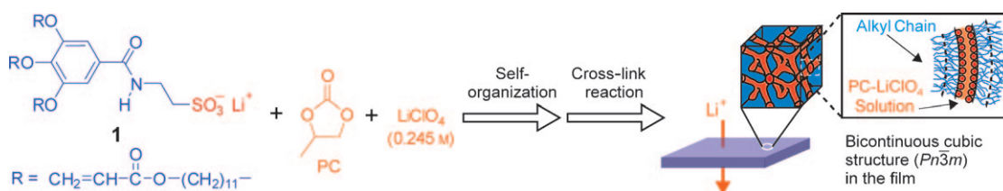
Figure 2. Preparation of nanostructured films having 3D interconnected ion-conductive pathways. [9]
